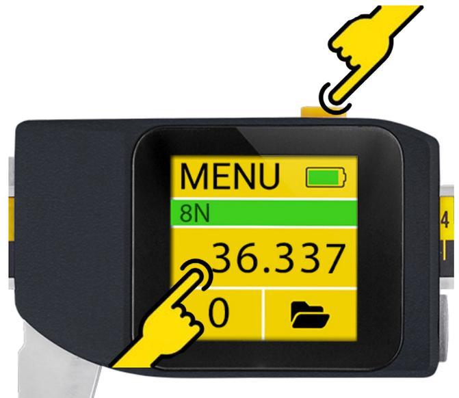
MICROTECH COMPUTERIZED INSTRUMENTS have **USB HID** data output to transfer Data direct to any compatible operation systems and applications in keyboard mode.
