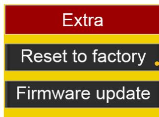
Push 10 times to RESET device to factory settings
