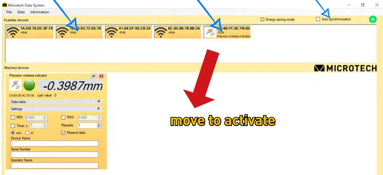
Select Filtering device mode in Connection menu to view only MICROTECH instruments in Available devices area
