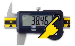
In economy mode the data transfer is carried out only by pressing the button It is necessary to activate **ECONOM** mode (Energy saving mode) on main screen
