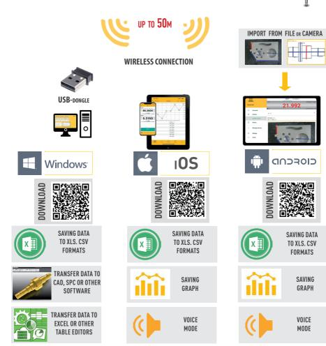
DATA TRANSFER DISTANCE FOR INTELLIGENT INSTRUMENTS •All MICROTECH Intelligent instruments has internal memory. You can collect data to memory and when it will be neccesary transfer all data to the peripheral device with no data loosing. •It's possible transfer data, like in Wireless instruments up to 15 m or up 50 m with external antenna •USB port can be used to transfer data directly to Windows PC
